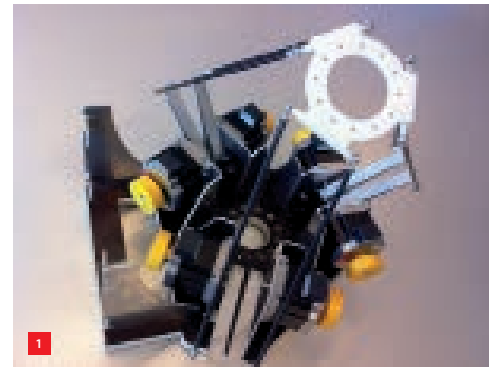
1 The HUniplacer is a delta robot.
